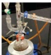
In a steam distillation, the essential oil of a plant is isolated as it co-distills with water.
